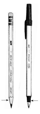
Insert pen or pencil into the jar lid to the point shown to create a hole with the proper diameter.
